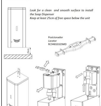
Open the unit with the provided key Remove the soap tank locator and the soap tank with the valve Remove the mechanism
